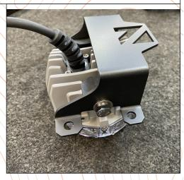
Step 6) Insert the mounted light into the bumper from the back side of the bumper.
