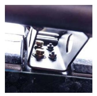
14. The **LMI** Light Bar has a number of light mounting slots that set the light to light mount spacing for you. See the Product Dimensions section below for details. After you have installed lights in the orientation of your picking, there are several zip-tie mounting locations that will assist you in routing the wire harness.
