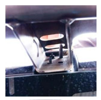
8. Drill four holes in locations marked in the previous step using a 3/8 inch drill bit. Take caution to ensure that the holes are drilled in the correct location, failure to do so will cause problems during installation.
